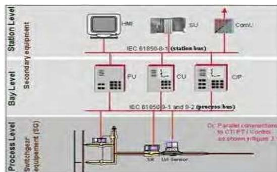
Fig 1 substation automation levels
