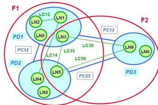
Fig 5 flexible functionality of LNs in different IEDs [7]
