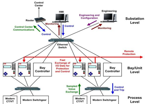
Fig 1 substation automation levels based IEC61850
