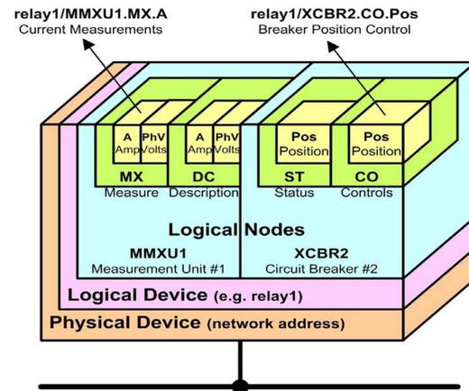
Fig 5 Object Oriented model in IEC61850
