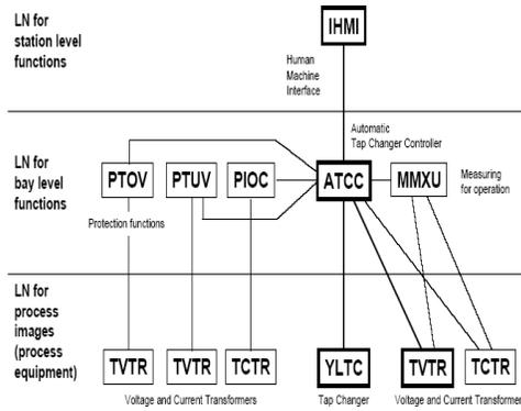
Figure 10 LN in different level
