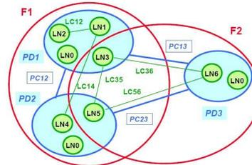
Figure 8 flexible functionality of LNs in different IEDs
